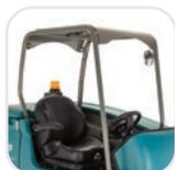
**Overhead guard** protects operators from falling objects.
